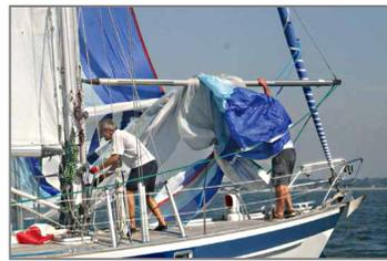
Handling systems come down to a choice between spinnaker socks and top down furling systems. Socks are simple and work well particularly on spinnakers with big girths. Top down furlers work but can struggle as the girths get bigger. The work well on smaller, flatter sails. Big width up high is still tough to get furled tightly and reliably. Top down furlers also need clearance between headstay and furled sail. A sprit really helps. A proper torsional rope is critical. Expense is higher.
